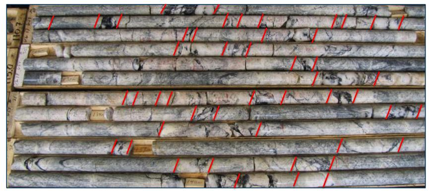
Dip of shearing -60 degrees / Angle of the hole -57 degrees
