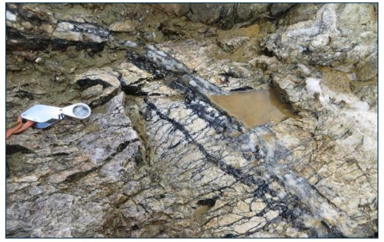
QTP-VG extension veining with tourmaline bleeding along shear fractures
