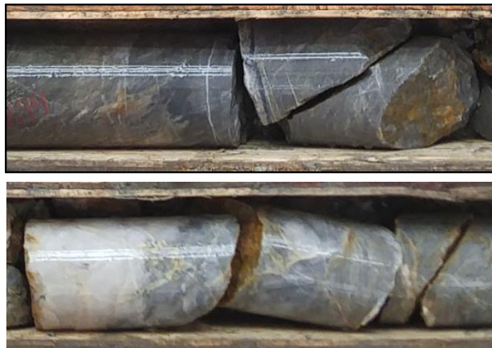
BV17-59: 52.5-53 m, quartz biotite schist and quartzite with veining
