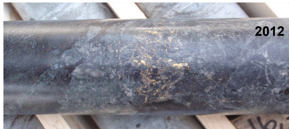
Diamond drilling ROM0011: 6 m @ 617 g/t Au
