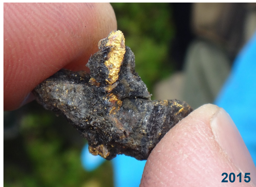
Diamond drilling ROM0011: 6 m @ 617 g/t Au
