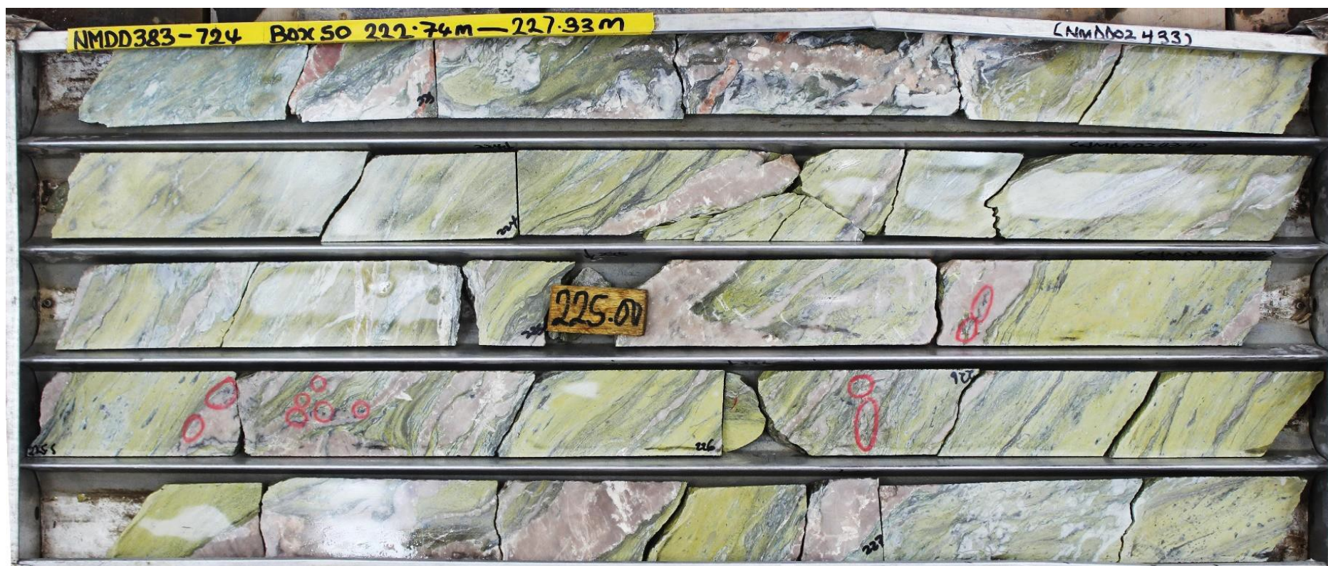
Cut drill core containing visible gold (red circles) within altered volcaniclastic rock unit
