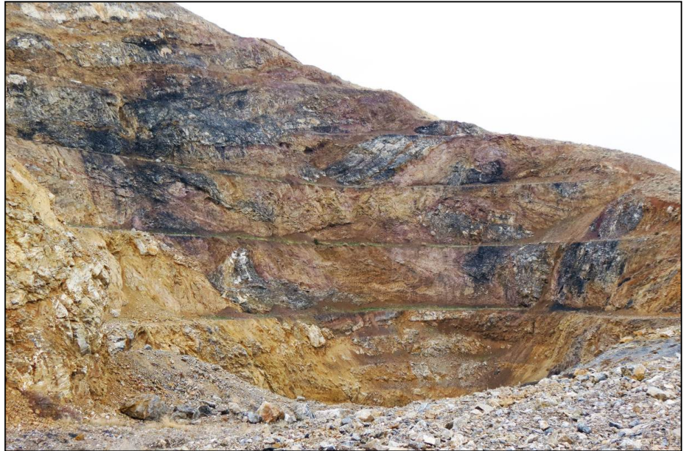
Low angle imbricate fault zone in the Tallman pit
