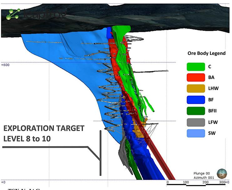
Spatial relationship between the mineralized zones at Pilar Mine in an east-west cross section (looking north).
