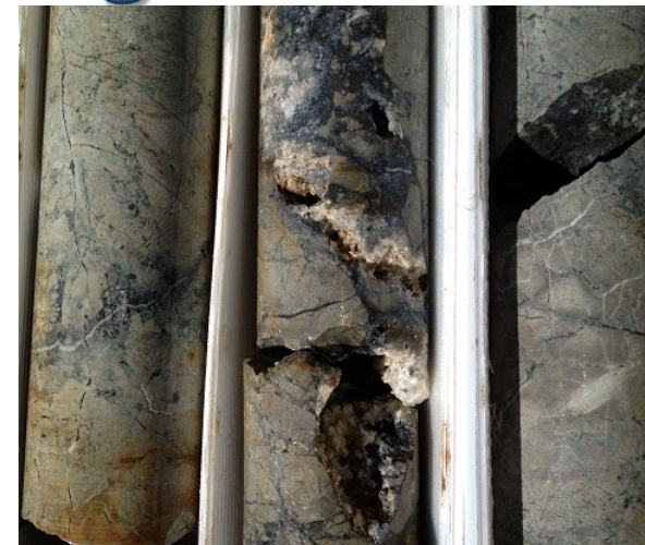
CAM12-02, 233m; Quartz-calcite and sulfide veining in hornfelsed sediments
