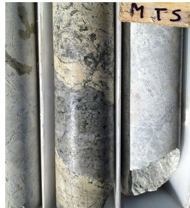
CAM12-02, 167m; Silica, clay carbonate altered brecciated hornfels sediment containing pyrite and dark silver minerals
