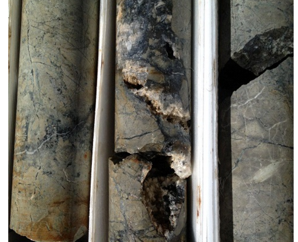
CAM12-02, 233m; Quartz-calcite and sulfide veining in hornfelsed sediments
