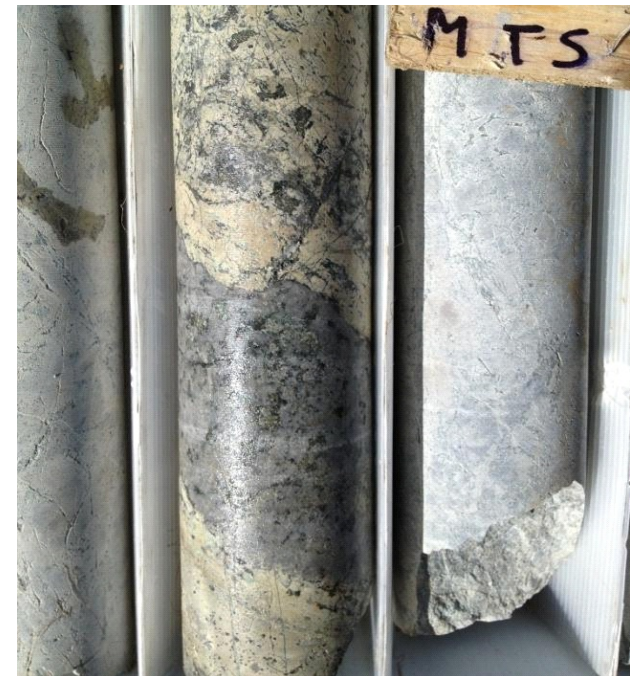
CAM12-02, 167m; Silica, clay carbonate altered brecciated hornfels sediment containing pyrite and dark silver minerals
