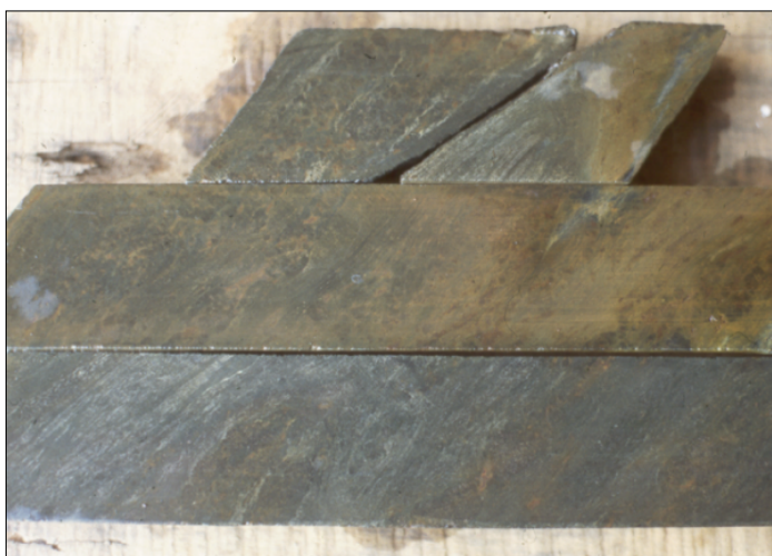
DH 96-08 Gold-bearing Chlorite Zones with Sulphides.
