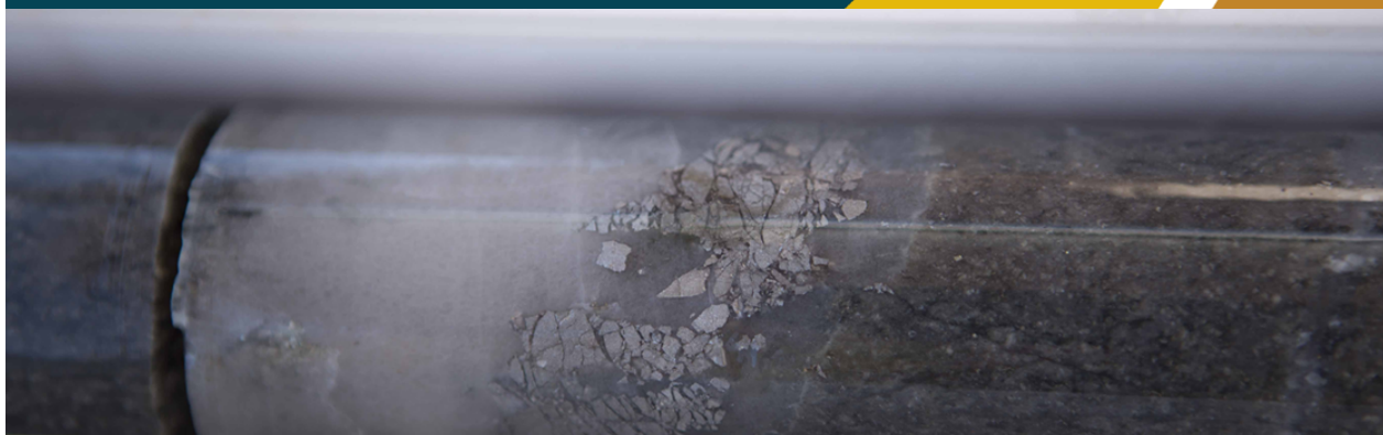
Gruyere drill core, 14GYDD0008 – Arsenopyrite vein
