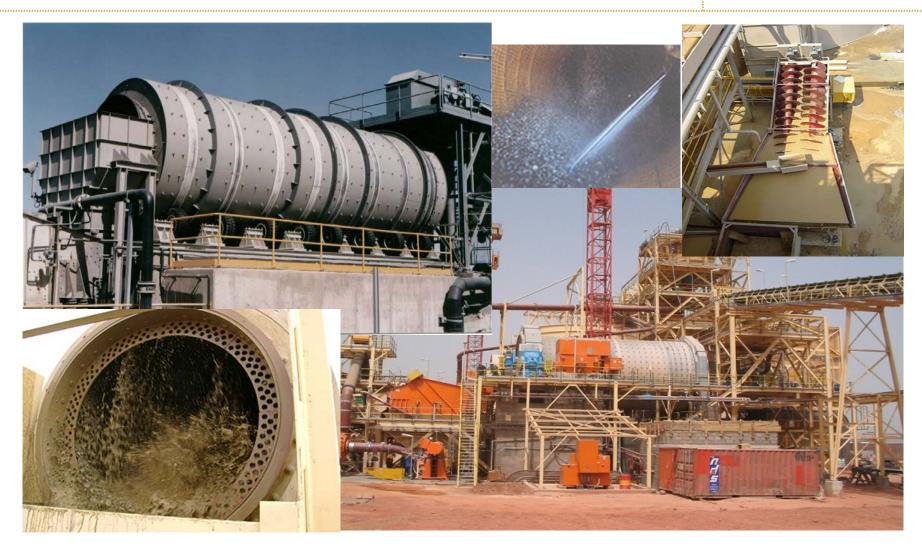
Up to 65% sent to ALC without milling, improving heap leach percolation and bringing forward gold recovery.
