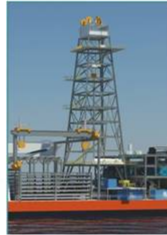
Derrick and Draw Works (riser handling equipment)
