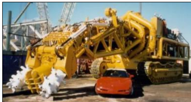
Second generation 200 ton offshore diamond mining machine, DeBeers, Namibia. Image courtesy Marine Minerals Pty
