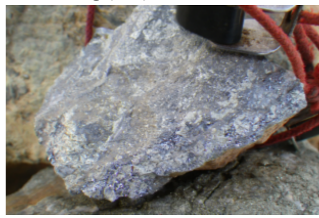
Porphyry Cu-Au target at depth Qtz + Cu oxide Stockwork
