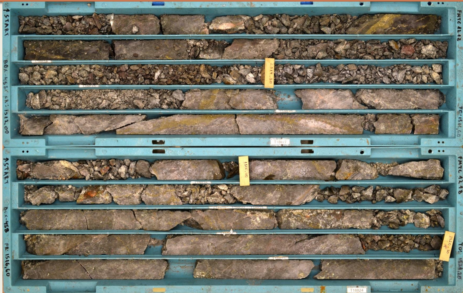
Drill Hole FMTC1218, 1512-1521m: 1.07% CuEq (0.92% Cu and 0.26g/t Au) Tectonic breccia and quartz altered andesite with disseminated pyrite - chalcopyrite
