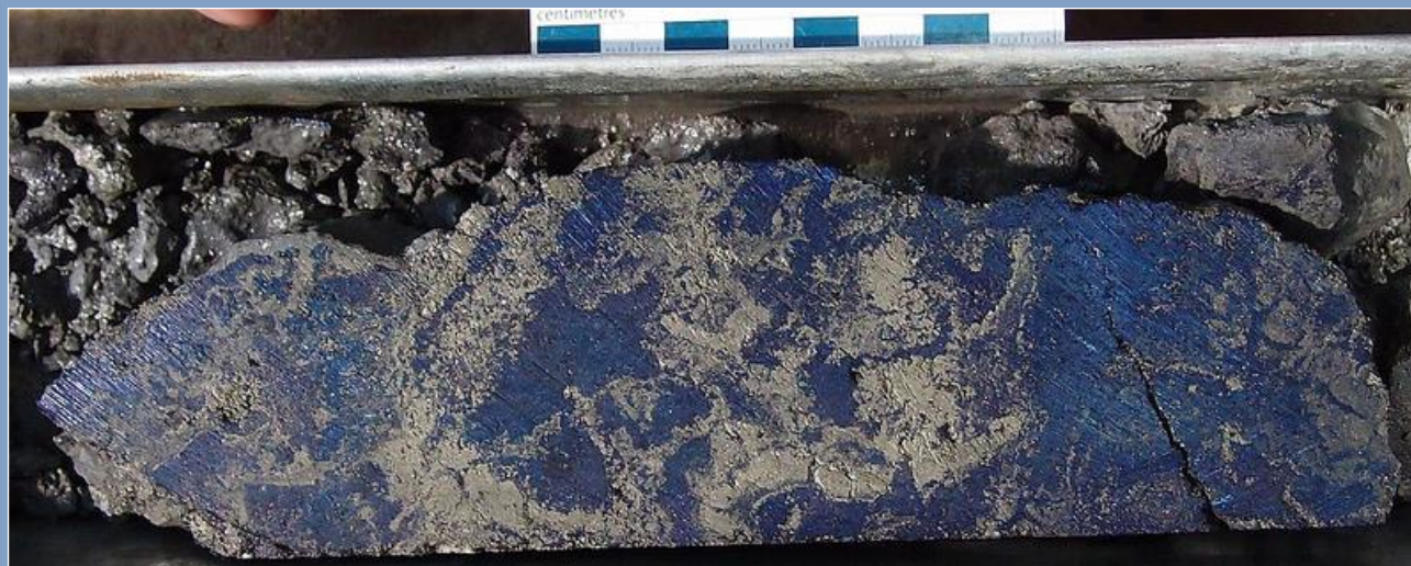
FMTC 1213 Drill core specimen. 508-509m 36.51% Cu, 8.50 g/t Au. 41.61% CuEq
