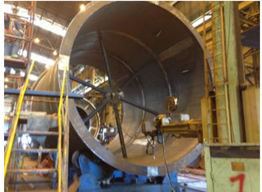
Circumferential welding of the Mill Shell strakes and flanges
