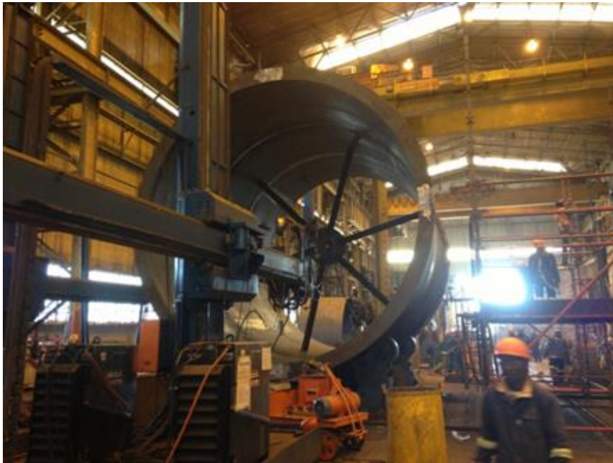
Circumferential welding of the Mill Shell strakes and flanges
