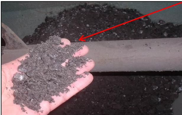
Mt. Todd Ore: Single-pass HPGR product from testing
