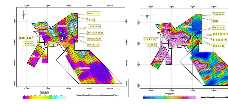
Resistivity lows indicating continuity of structure, highs indicating silicification
