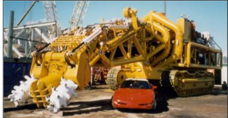
Second generation 200 ton offshore diamond mining machine, DeBeers, Namibia. Image courtesy IHC MMP
