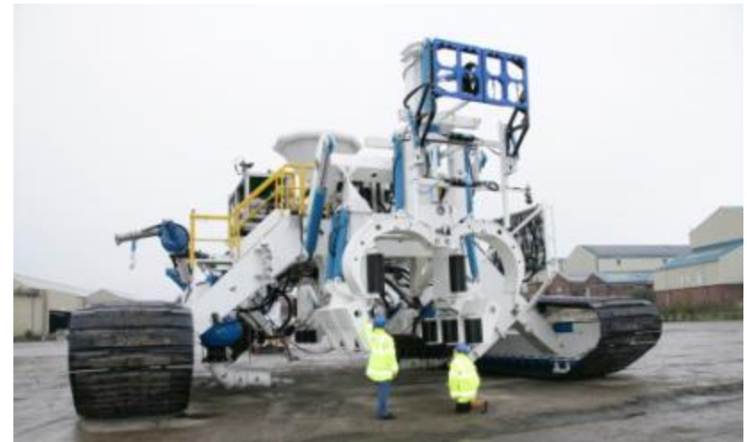
Sub-sea trenching vehicle designed and built by SMD. Image courtesy SMD
