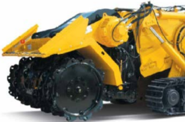
Onshore Continuous Miner Cutting Head
