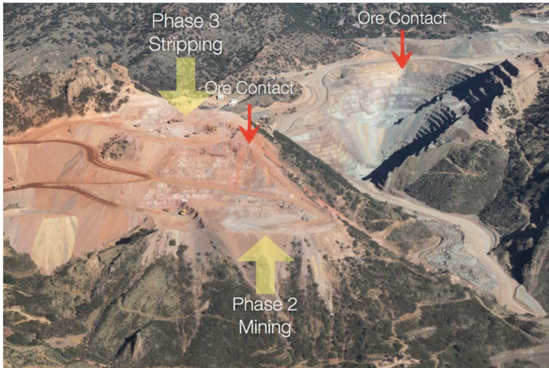
Aerial photo showing mining phases. Primary ore contact (western bounding fault) marked by red arrows. March 19, 2010
